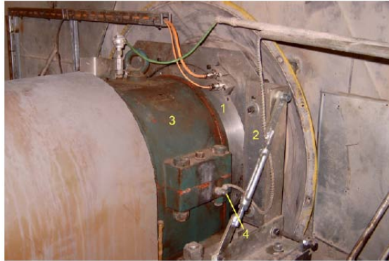
Large radial fan with installed balancing unit 1 Balancing ring, 2 Stator mounting adapter, 3 Bearing housing, 4 Vibration sensor
